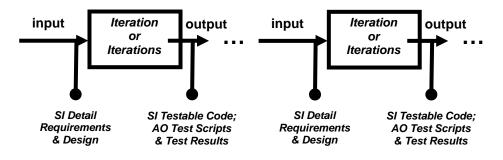
**Figure 3**. Iterative SDLC with Waterfall Overlay, called "IterFall" by the authors. In this figure, one or more iterations (sprints) would produce a software release that the acquiring organization or a third-party can test. Here, "SI" denotes system integrator (prime contractor) and "AO" denotes acquiring organization.
