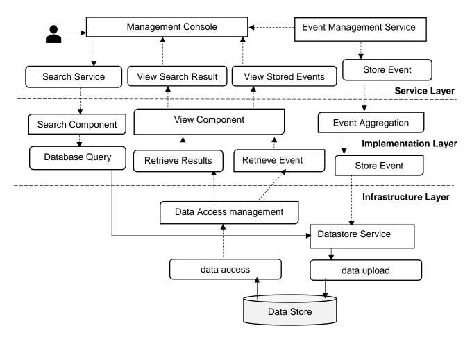
Figure 2 Layered software architecture
