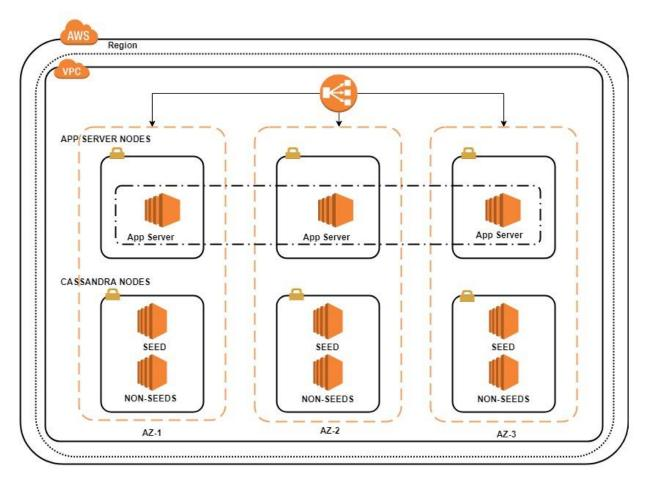
Figure 3 AWS Deployment Diagram
