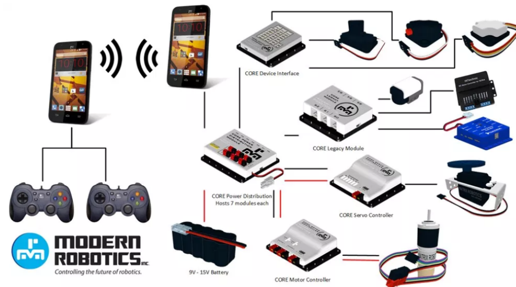
Figure 2. The control system of an FTC robot and its subsystems consisting of joysticks (used by drivers), Android smartphones with pre-loaded software programs, core components (e.g., external sensors, motors, power, etc.) to detect and control FTC robot [5]
