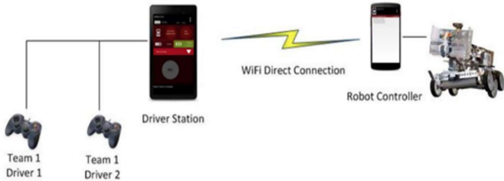
Figure 3. The control system of an FTC robot and its subsystems consisting of joysticks (used by drivers), Android smartphones with pre-loaded software programs, and core components (e.g., external sensors, motors, power, etc.) to detect and control FTC robot [5]
