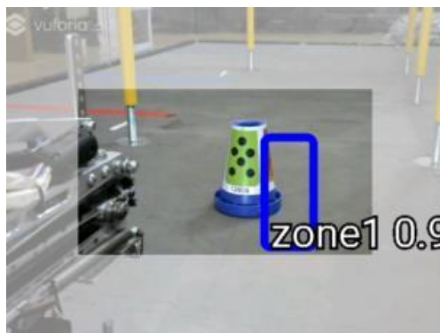
Figure 10. Illustration of signal cone sleeve pattern detection using TensorFlow machine learning
